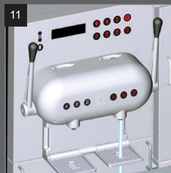
Automatic external rinsing: An approximately 25-second automatic rinsing of the milk system will begin 5 minutes after the last milk-based beverage preparation.
