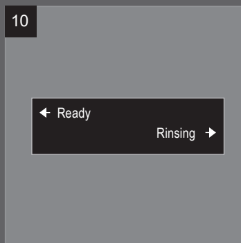
Automatic internal rinsing: An approximately 20-second internal rinsing of the milk system will begin immediately after each milk-based beverage preparation.
