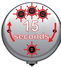
Descale machine (see page 16-17). The alarm first appears when the machine is switched on and repeated every hour.
