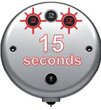
Change filter (see page 21). The alarm first appears when the machine is switched on and repeated every hour.
