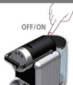
**2** If alarm is repeated after switching ON/OFF several times: descale machine (see page 16-17).
